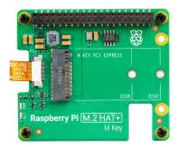
The Raspberry Pi M.2 HAT+ enables you to connect M.2 peripherals such as NVMe drives and Al accelerators to Raspberry Pi 5's PCle 2.0 interface, supporting fast (up to 500 MB/s) data transfer to and from NVMe drives and other PCle accessories.
