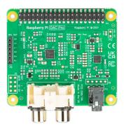
Raspberry Pi DAC Pro is our highest-fidelity audio HAT, and is compatible with any Raspberry Pi computer that has a 40-pin GPIO header. With the Texas Instruments PCM5242, the DAC Pro provides an outstanding signal-to-noise ratio (SNR) and supports balanced/differential output in parallel to phono/RCA line-level output. It also includes a dedicated headphone amplifier.
