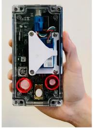
The 2B Technologies Personal Air Monitor (PAM) uses air pollution sensors in a compact, portable package. It maps and graphs pollution levels in 2B Tech's free Smartphone app, with option for uploading data via cellular service to the 2B Tech Data Portal.
