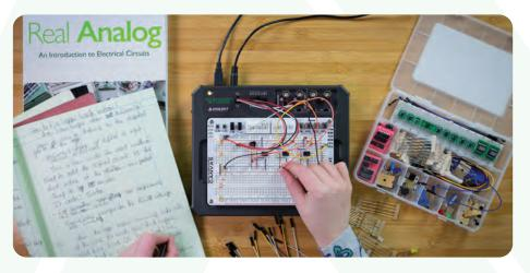
The Analog Discovery Studio is a fully-functional portable test and measurement device that can turn any cross-functional space into a pop-up electronics laboratory. Equipped with 13 instruments including an Oscilloscope, Logic Analyzer, Spectrum Analyzer, Waveform Generator, and more; the Analog Discovery Studio provides an entire stack of benchtop instruments with a convenient breadboardable interface, perfect for enabling circuit design anywhere!
