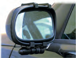
D x mirror antenna for unobtrusive placement during road tests
