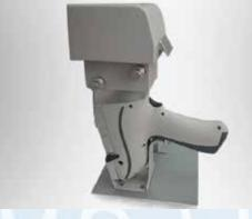
Use a laboratory stand to prevent X-Ray scattering when analyzing small objects or light matrix samples.
