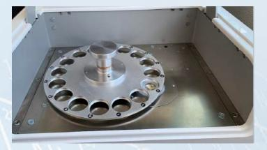
The automatic 16-positions sample changer coupled with the fast measurement increases the productivity of your lab up to 1000 samples per workday.
