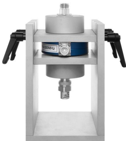
Picture 2: TBCP4-CAL RF current probe calibrator
