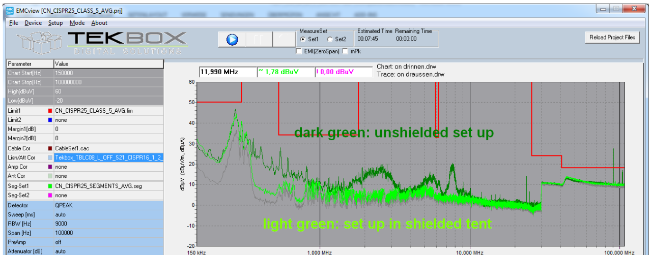
Picture 6: CISPR 25 conducted noise measurement; DUT powered
