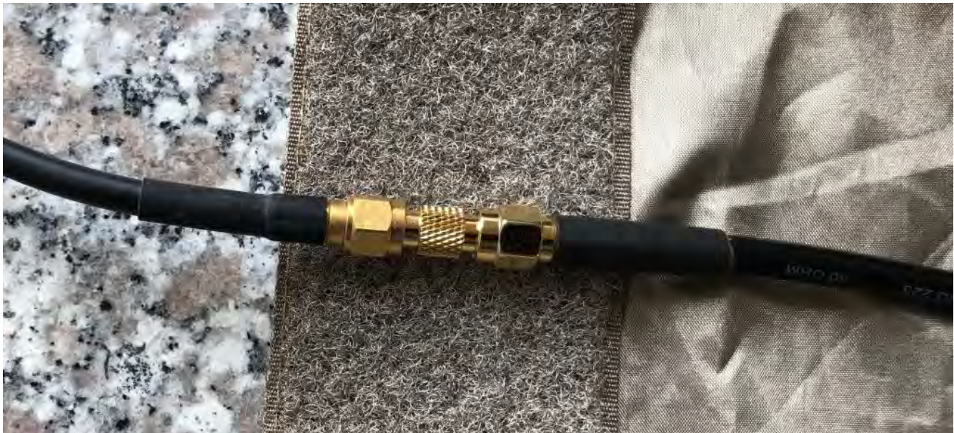
Picture 9: feed through using coaxial adapter
