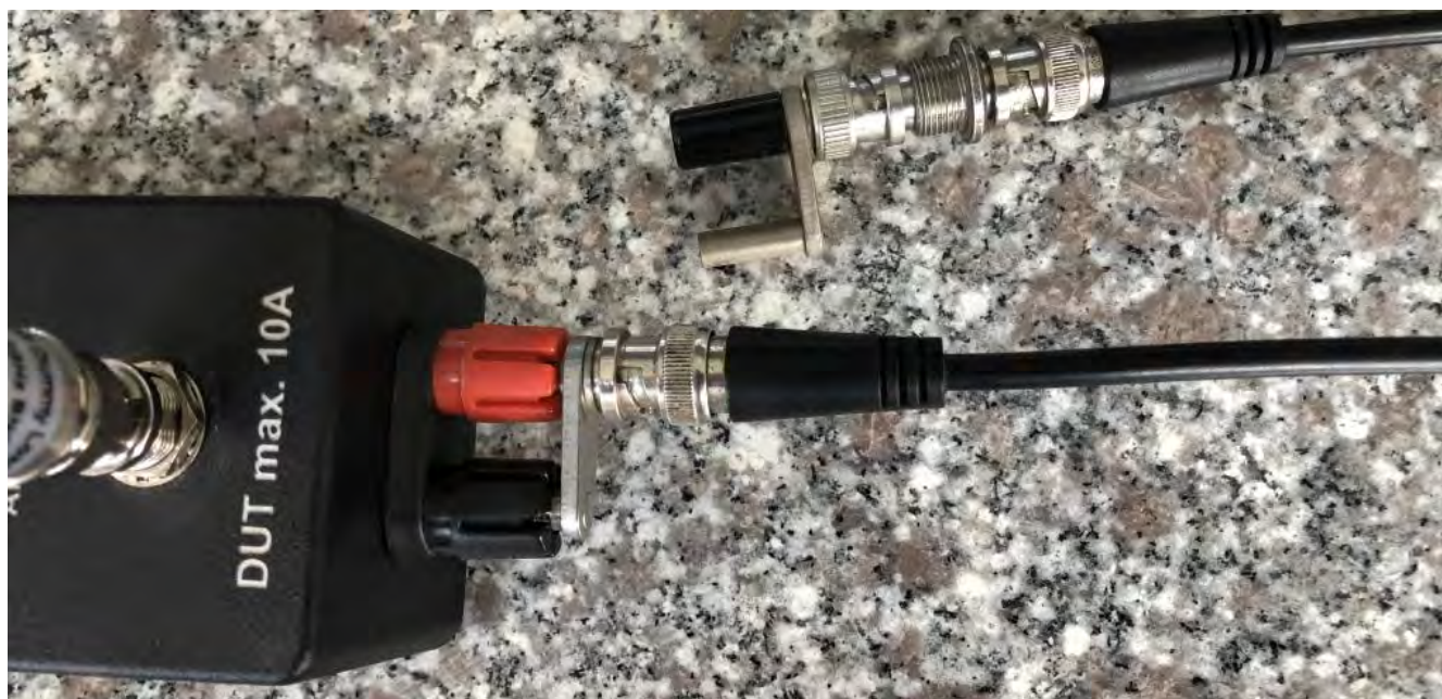
Picture 18: using banana to BNC adapters and a BNC cable as shielded supply line
