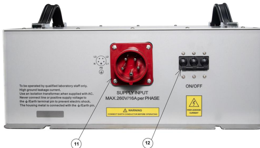
Figure 6 – Rear panel layout
