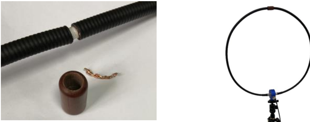
Picture 2: using corrugated coaxial cable to build a loop antenna
