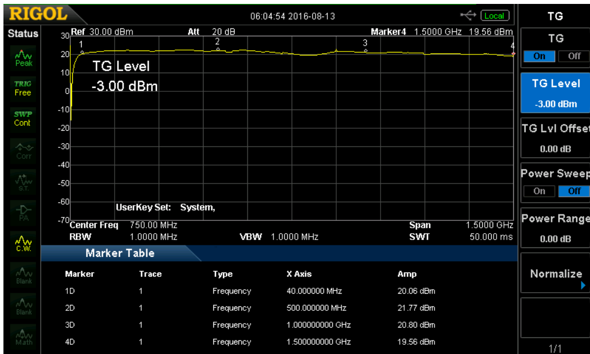
Picture 6 – output power of the TBMDA1, CW, driven by the DSA815 tracking generator set to -5dBm
