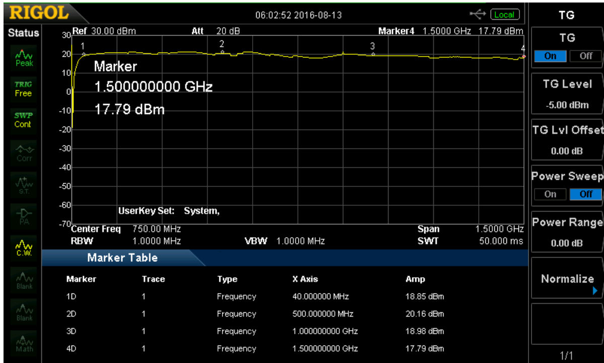
Picture 6 – output power of the TBMDA1, CW, driven by the DSA815 tracking generator set to -5dBm
