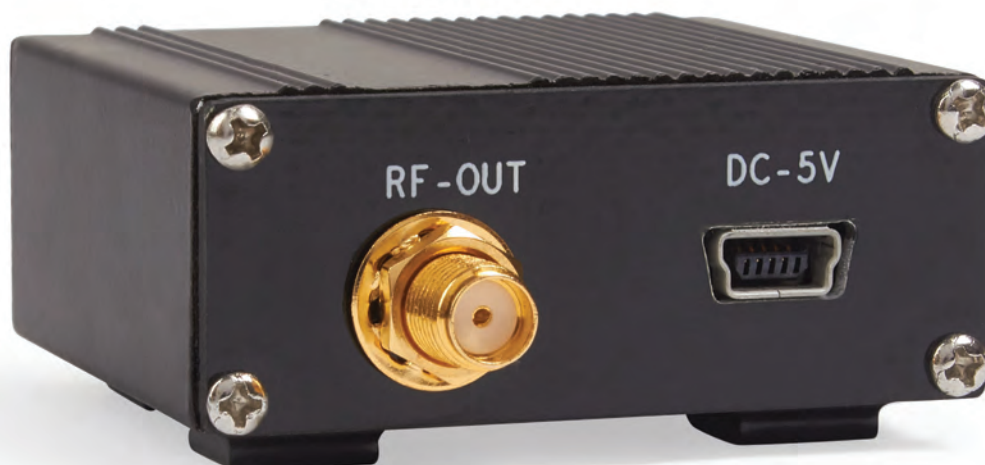
Picture 2 – TBHDR1 wide-band RF pre-amplifier, rear view
