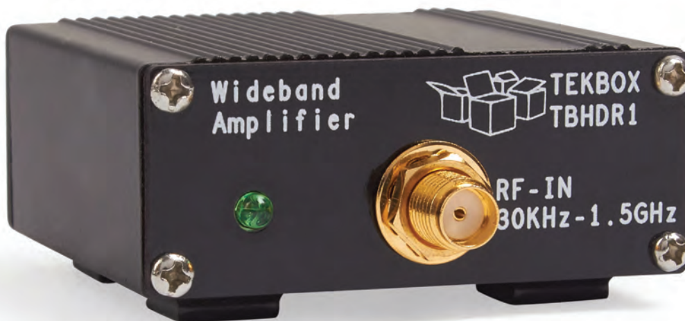
Picture 1 – TBHDR1 wide-band RF pre-amplifier, front view
