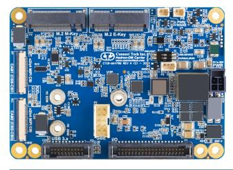
Hadron's design includes a wide input voltage, rich I/O set as well as locking IO connectors optimized for rugged environments.
