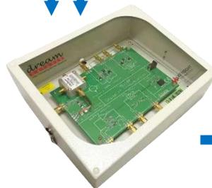
The digital RF communications kit requires two function generators to provide the IQ baseband signals.
