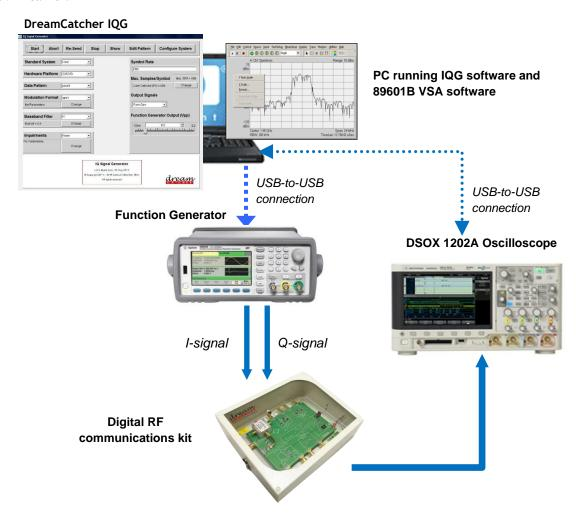
The digital RF communications kit requires two function generators to provide the IQ baseband signals. The low-frequency module contains a 10 MHz IQ modulator used to generate an IQ modulated RF signal, which is then analyzed by the VSA software on the oscilloscope.
