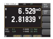
Standard Mode (Setting conditions and R+V measurement parameters)
