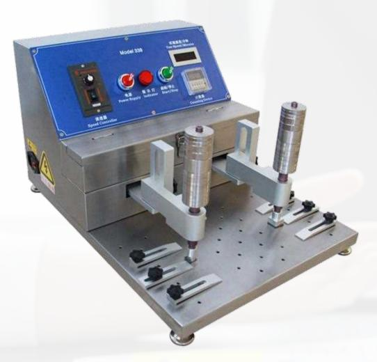
The friction testing machine is suitable for all kinds of non-conductor coating layers, all kinds of plastic products oil injection, silk screen surfaces for friction test, such as computers, mobile phones (P.D.A), MP3, CD/VCD/DVD, cordless phone, electronic dictionary, etc., the friction testing machine can also be used as LCD nod fatigue test and handwriting stroke test;
