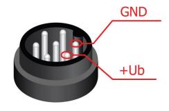
Sap flow measuring unit MicroSet 8X - female connector for DR26E wiring
