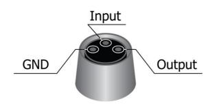
Standard M8 male connector cable wiring
