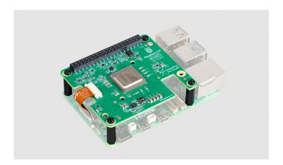
The Raspberry Pi Al HAT+ is an add-on board with a built-in Hailo Al accelerator for Raspberry Pi 5. It provides an accessible, cost-effective, and power-efficient way to integrate high-performance Al. Explore applications including process control, security, home automation, and robotics.
