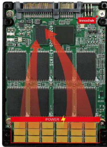
Figure 3: Diagram of 2.5" SATA SSD with iCell
