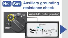
When measuring an installation with low grounding resistance, inadequate measurement sensitivity can interfere with measurement. The FT3151 lets you check the auxiliary grounding electrode S (P), too.
