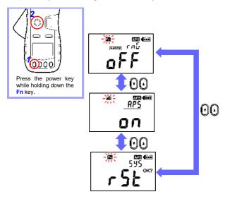
To exit sub-function mode, press the power key to turn off the instrument and then turn it back on.
