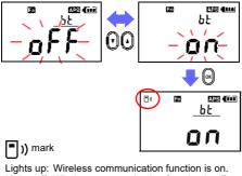
Lights off: Wireless communication function is off. Flashes: Performing wireless communication
