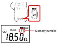
When the number of values saved in the instrument's memory reaches 2,000, the display will show "FULL," and you will not be able to save additional values. Delete unneeded values to free up space.
