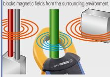
Minuscule leakage currents can be accurately detected since the meter is resistant to the effects of external magnetic fields.
