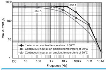
When measuring current close to the derating, allow a cool-down time of at least 10 times the time for which the current was input.
