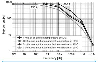
When measuring current close to the derating, allow a cool-down time of at least 10 times the time for which the current was input.
