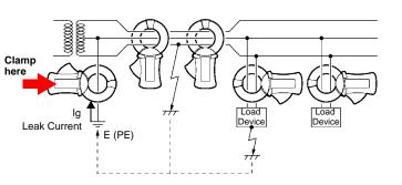
2. If current leakage is detected, further bundled measurements (clamping around bundled conductors) is employed to search from the source to the load side.
