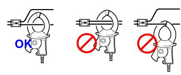
When making the phases of the measurement current and output voltage the same, clamp the jaws of the sensor onto the conductor so that the current direction on the clamp points in the direction of the load, and so that the conductor is approximately centered between the jaws. Make sure that the tips of jaws are fully closed.
