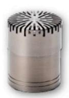
Low-frequency microphone especially designed for infra-sound measurements. Frequency range from 0.5 Hz to 20 kHz. Use the dedicated 26CG 1/4" CCP preamplifier in order to obtain the low frequency response.
