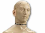
simulators, the IEC 60318-4 Ear Simulators or various  $\frac{1}{2}$ " and  $\frac{1}{2}$ " pressure microphones for binaural recordings. KEMAR accommodates for LEMO as well as CCP preamplifiers which are all electrically accessible from the connector panel on the back. Additionally, all CCP configurations are IEEE 1451.4 TEDS v. 1.0 compliant.
