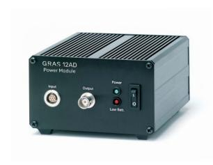
12AD is a 1-channel, battery-operated, microphone power module. It has a 7-pin LEMO 1B input connector for a microphone preamplifier and one BNC output socket. It can provide a polarization of 200 V for externally polarized or 0 V for prepolarized microphone cartridges.
