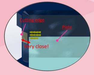
The area around the blade has a simple shape. This makes it possible to approach the wafers and glass plates close to the blade, making the collection easier.
