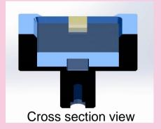
The boat section is the deepest compared to other Jumbo types. Then, the lower part of the blade is vertical and the corners are squared, so glass plates or wafers can be stably installed in the desired position.
