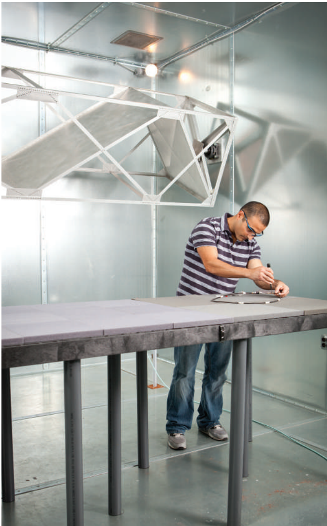
Mode stir RF-Shielding testing per IEC Standard 61000-4-21 Annex F
