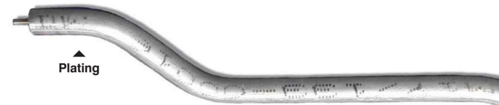
Copper and aluminum conductors are often plated for additional corrosion protection and solderability. The most common plating materials, tin and silver, are very soft and ductile.
