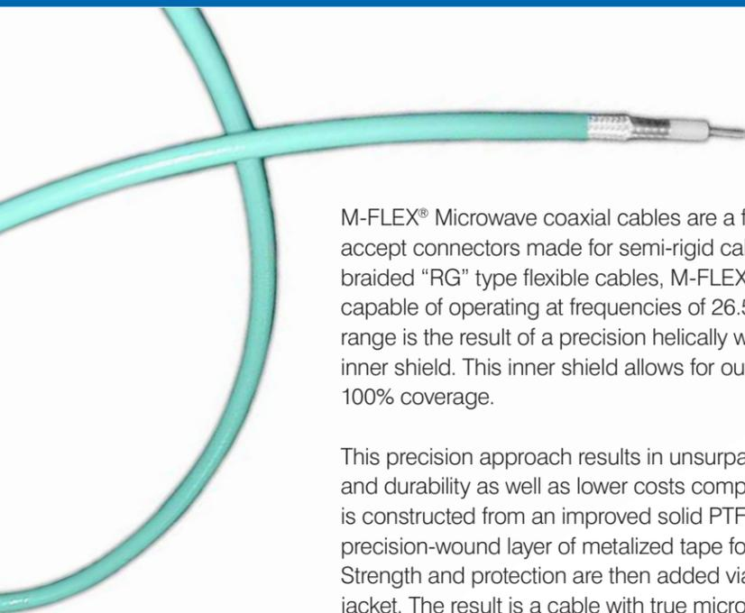
M-FLEX® Microwave coaxial cables are a family of flexible cables designed to accept connectors made for semi-rigid cable. Unlike other single- or double-braided “RG” type flexible cables, M-FLEX® cables are true microwave cables capable of operating at frequencies of 26.5 GHz. The extended frequency range is the result of a precision helically wrapped silver-plated copper foil inner shield. This inner shield allows for outstanding flexibility while providing 100% coverage.
