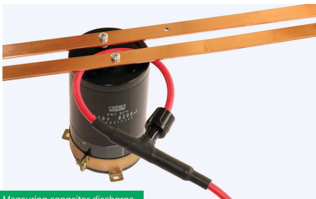
Measuring capacitor discharge
