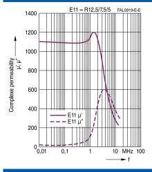
E11 offers a cost-efficient solution for high-frequency EMI suppression over nanocrystalline and NiZn ferrite cores in the frequency range of 30 MHz to 300 MHz. Curie temperatures above +150 °C qualify the material for automotive applications.
