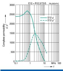
E12 provides flat  $\mu_i$  over the temperature with a Curie temperature above +170 °C.
