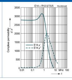
E13 and E14 as new materials bring together high saturation and high impedance up to 30 MHz for hightemperature applications. The Curie temperature exceeds +220 °C for E13 and +255 °C for E14.
