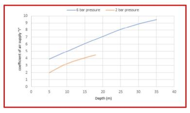
Variation in the pump flow rate according to the operation depth. This graph is referred to 2 m hydrostatic head and 6 bar pressure of compressed air supply
