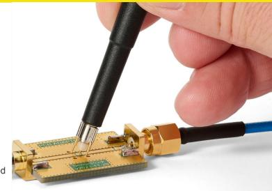
The SQG-series includes exchangeable fine-pitch spring-tipped test needles, ensuring reliable contact with small or delicate components.
