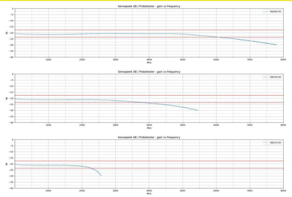
\*Graphs shows typical performance of an actual measured probes from volume production. *SPID (Sensepeek probe ID): SQG15-DC B26083, SQG30-DC E45F44 and SQG60-DC C50260*
