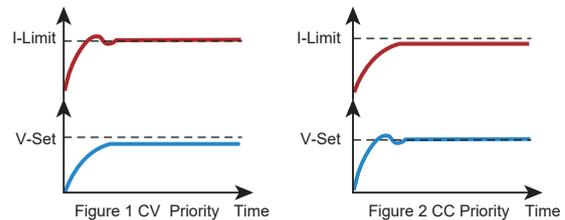
As shown in Figure 2, when it needs to reduce current overshoot during testing or the component to be measured is low impedance such as in the battery charging scenario, the current priority mode should be used to obtain a fast and smooth rising current.
