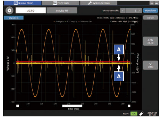
Setting of PD threshold
