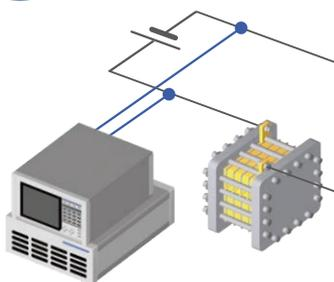
Connect the SOURCE MODULE to the cell's power source terminal with the SOURCE CABLE. The SOURCE MODULE applies AC current for measurement.
