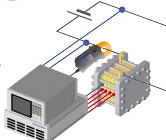
Attach the current sensor to measure the current. Then, connect the SENSE CABLE to the cell to measure the voltage (both connected to the SENSE MODULE)
