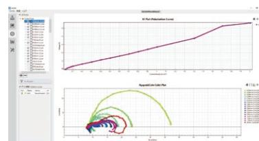
Start the measurement the I-V curve and Nyquist plot will be displayed in real-time during the measurement.
