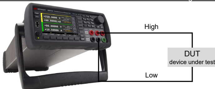
Same measurement using an SMU
