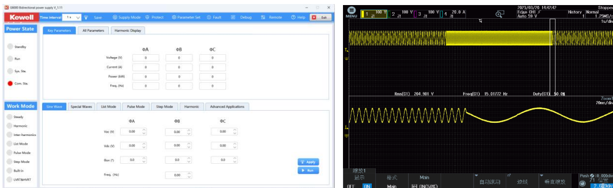
Fig. 4-5 DC+AC @200Vdc superimposed with 50Vac, frequency varying 15Hz -100Hz -15Hz
