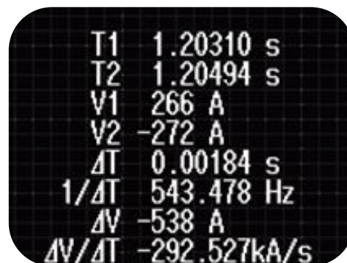
Switching time \leq 2\text{ms} (-90% ~ +90% switching)
