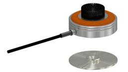
When the 147AX microphone set is placed over the mounting disc, a center guide ensures that the microphone will be attached and centered to the disc correctly once the magnetic force kicks in. In this way, it is easy to mount in difficult-to-access locations with no loss of placement accuracy.
