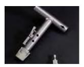
When either a 5 gram or 25 gram disposable En Core Sampler arrives at the laboratory, attach it to the Extrusion Tool, engage the plunger and push the sample into an appropriate vial.
