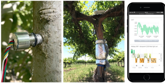
FloraPulse subscription. Includes the sensor probe, installation kit, cellular data and visualization.
