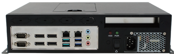
Rear I/O (Based on MI989 I/O)
