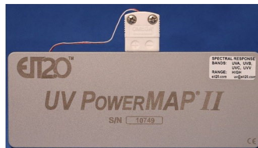
Top: Instrument with thermocouple
